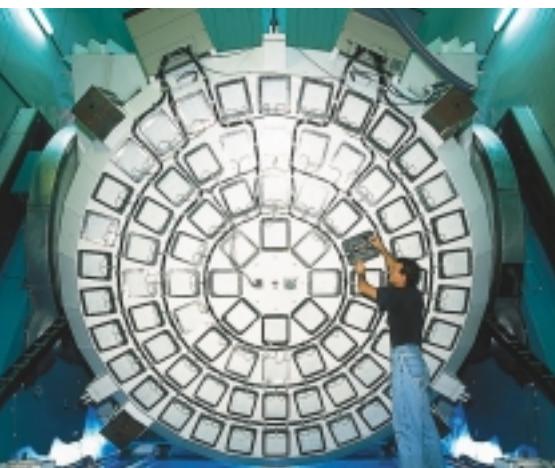
Figure 5.29 The New Technology Telescope (NTT) is one of the telescopes pioneering adaptive optics. Its mirror is constantly deforming in time with the atmosphere to remove the twinkling effect.
